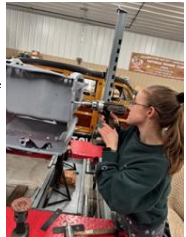
Removing some spotwelds
