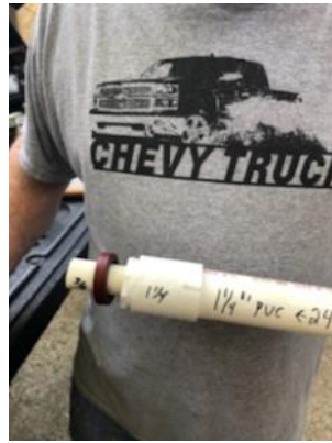
B. Grease 3/4" PVC so Seal Slips on
