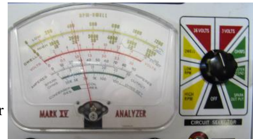
Cranking voltage at coil did not vary
