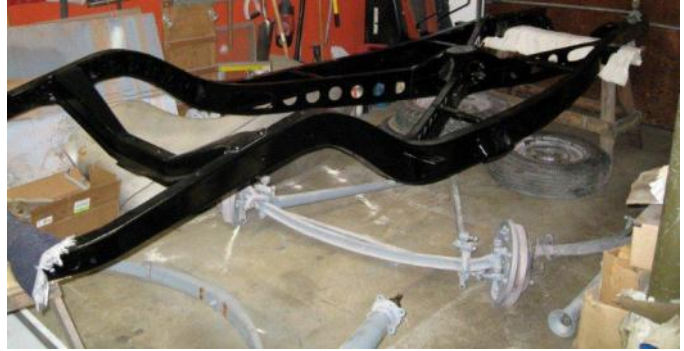
The bare frame before work begins on the chassis
