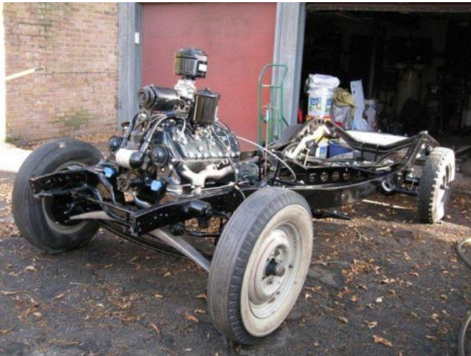
The completed chassis ready to be mated with the body
