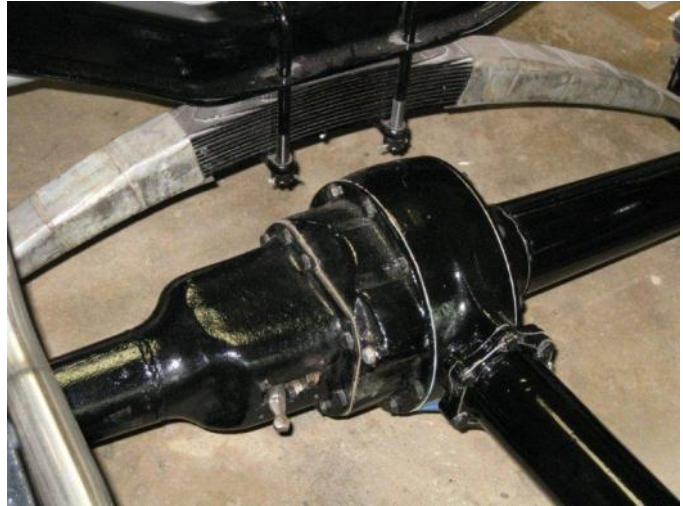
Mounted Columbia with correct left axle housing
