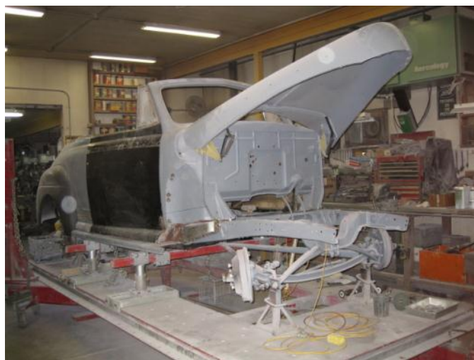
Body work in progress with new convertible doors
