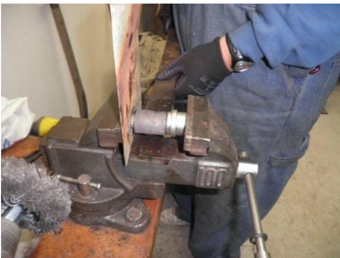
Pressing out the bushing using a vice
