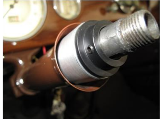
The new bearing assembly slides over the steering shaft – note the set screw
