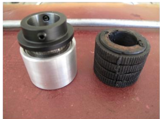
New precision bearing assembly compared with old worn bushing
