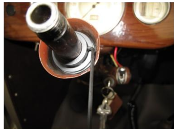
New bearing in place, Allen wrench used to securely tighten the two set screws
