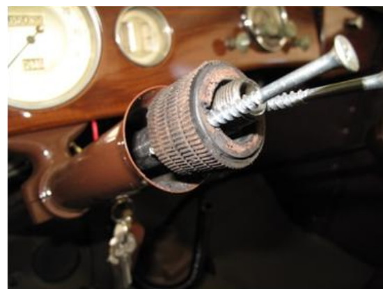
Removing old bushing with the aid of deck screws
