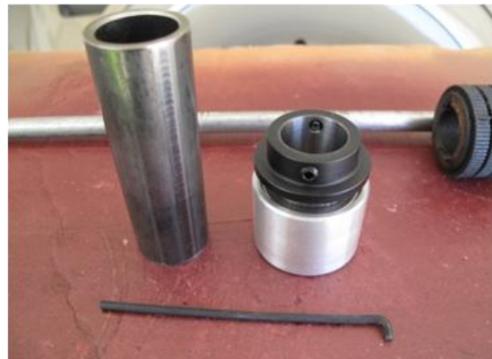
Bearing kit includes two-piece needle bearing, driving tool, and cut-off Allen wrench.
