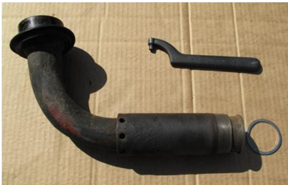
Filler tube, lead seal on right, spanner wrench above
